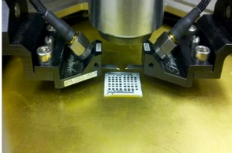
Figure 44. TRL experimental set-up
